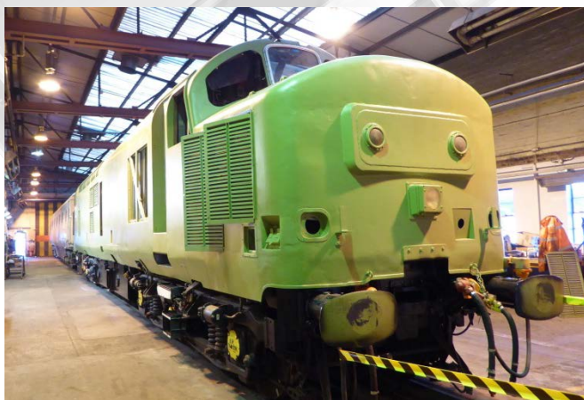
37800 in green undercoat nears the end of its re-build in Leicester locomotive depot.
