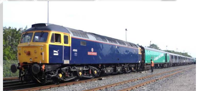
Locomotive haulage of a class 321 EMU using T5 translator vehicles. ROG's 5Z21 service from Ilford arrives at Old Dalby.
